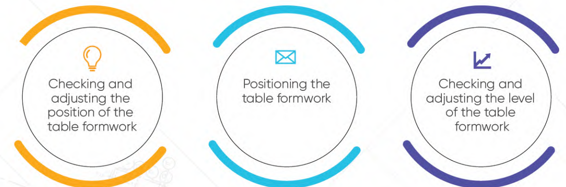
Figure 2.10. Crucial elements in setting out, alignment, and level check (BCA, 2012)
